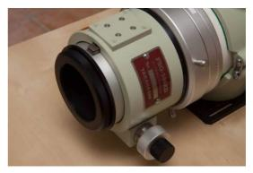
Install the Takahashi focal reducer (x0.73) on the telescope. Tighten it gently.
