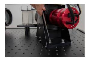
The camera lens must be as close as possible from the prisms holder, to prevent any vignetting (light loss).
