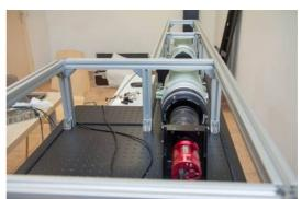
To make an image of the fiber with the camera at this position, we must send back the beam coming out the telescope #1 towards the telescope #2. To do this, put the flat mirror (only used during the tuning), at the end of the telescope #1. By doing this, we make a symmetrical system, and we should see exactly the same image of the fiber.
