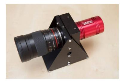
A simple way to check this is to put the camera module on the optical bench, and measure the height of the optical axis (center of the lens) above the bench. It must be 102mm.
