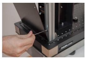
Put first the bottom screws (in the optical bench). If not already done, make a slot in the gasket (with a cutter) at the position of each screw.
