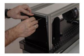
Install Bosch spring nuts in the Bosch profiles, matching each holes in the cover. Make sure each spring is aligned with the hole.
