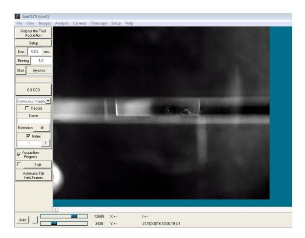
When the tuning is optimal, tighten gently the telescope #1 plate on the optical bench.
