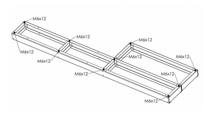
Put the two optical benches on a flat and clean surface (table), with the faces with many holes towards the ground. Position the benches like on the picture (make sure that the adhesive tape on the top face are matching!) :
