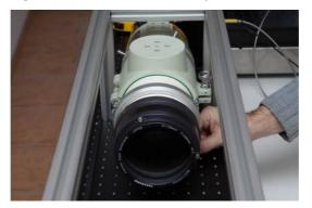
The end of the lens (body of the focal reducer) must be at a distance of 69mm from the light spot on the input mirror.
