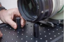
Install the flat tunning mirror at the end of the telescope #1. Attach it gently with adhesive tape, and make sure it is well stuck on the telescope body.
