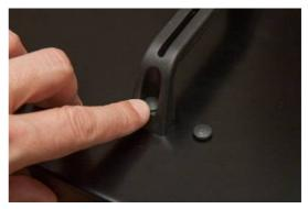
Put Bosch spring nuts in the Bosch profiles, matching all holes in the covers.
