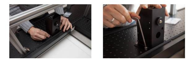
At the end, you can check that the fiber axis is at 102mm above the bench. There is no optical test to make at this stage.
