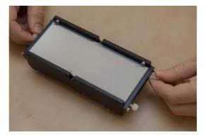
Gently tighten the 3 plastic screws BELOW the mobile holder. This will push the grating towards the three screw heads. This must be done keeping the grating surface towards the roof.
