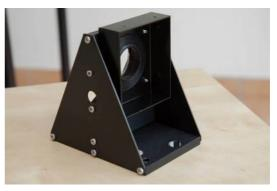
Make sure that the camera plate is perpendicular to the camera base (use the set square). If it must be corrected, untighten the side screws, and adjust the plate.
