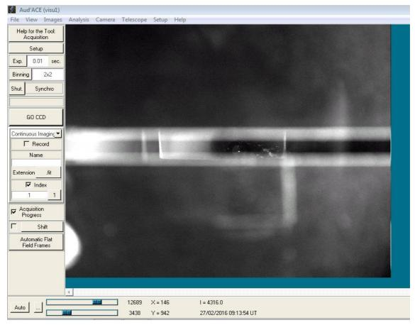
In this case slightly rotate the telescope #1, without losing the focus ; use the tuning tool to lock its axial position, and add screws on the side of tuning tools to help making a very precise tuning. It is very sensitive : you can use the side tools (along the telescope plate) to help you.
