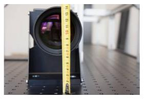
Put the CCD vertically (Atik logo on the top in our case). Tighten the camera adapter in the holder using the three headless screws at 120°.
