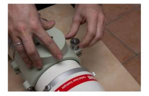
Remove the adapter rings at the rear end.
