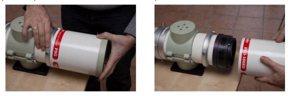
Remove the rear cap (from the focal reducer). Put the collimator assy on the bench, at a distance of 138mm from the telescope #1 (it is symmetrical from the input spot on the mirror :  $2 \times 69$ mm). Make sure that the lense axis is exactly parallel to the bench edges (visual control is enough). Attach the module to the bench with four M6x16 screws, with one flat washer and three spring washer for each.
