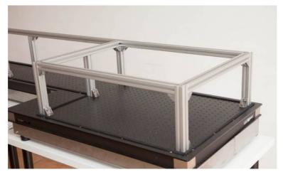
Add a bracket on the middle vertical element. Use the precision steel set square to make sure the angle is right.
