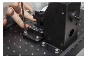
Put the horizontal and vertical tuning in nominal position. The final and precise angle will be tuned later in the process.
