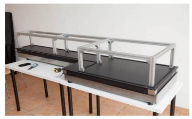
When all elements are in place, check all right angles and tighten the Bosch brackets. Make sure that all screws are tightened. Then tighten the special brackets on the optical bench. At the end, the structre is very strong.
