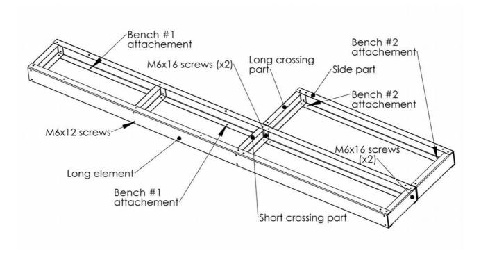
Put 2 M6 screws at each end of the crossing parts. Make sure that the result complies to the above picture. Specially, the 8 mentionned holes must be at the right place.
