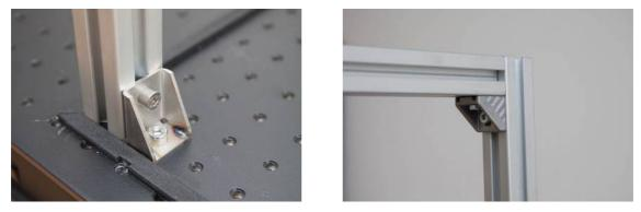
Start with the longest vertical profiles (240mm, 5 parts), attached to the optical bench. Use only one special bracket for each vertical Bosch profile. The
