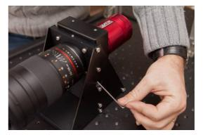
Plug the power supply cable, then connect the USB cable to the acquisition PC. Check that you can acquire some images.
