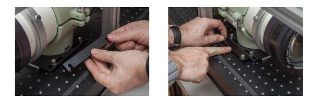
Use a third tuning tool to make a fine focus tuning (attached to the bench with two M6x16 screws & washers, and using a M4x40 screw for the tuning)
