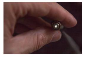
Remove the fiber connector cap and plug the fiber in the FC connector. Take care of the index in the connector.
