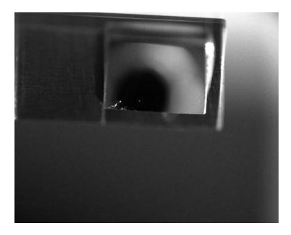
Precisely adjust the focus of the telescope in such a way that the fiber image is as small as possible. Images must be take in binning 1x1, and the fiber image must not be saturated. With 50 $\mu$ m fiber and Atik 460EX camera, the FWHM should be around 3,9 pixels.
