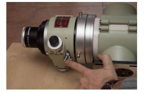
Remove the telescope cap, and the dew shield from the telescope. To remove the dew shield, tighten the two screws, then unscrew the whole shield. Keep the cap and the dew shield in a safe place (no more needed in the eShel+).
