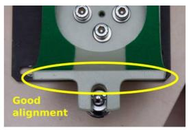
Put the Takahashi telescope #1 in its holder ring. Let 10mm from the ring (this will be useful for making a good alignement later on).
