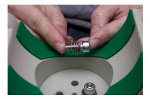
Make sure the telescope ring is perfectly parallel to the holder.
