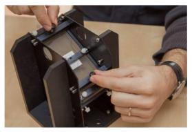
To move the spectrum vertically, rotate the camera holder around a vertical axis, close to the front lens. Keep in mind that the whole light beam coming out the last prism must be catched by the objective lens.
