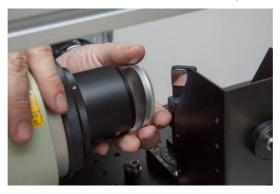
Put 4 M6x16 screws (plate washer + spring washer for each) to attach the telescope on the optical bench. The optical axis of the telescope is at
