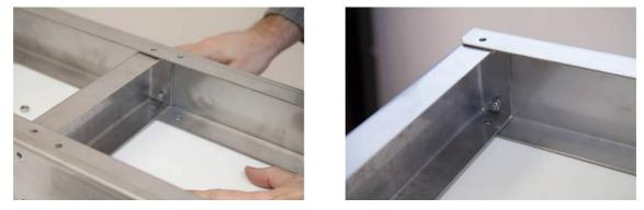
Put 10 M6x12 screws on the top face of the structure (make sure it is like on the picture below ; if needed, return the structure). Leave the 8 holes for benches attachement free.
