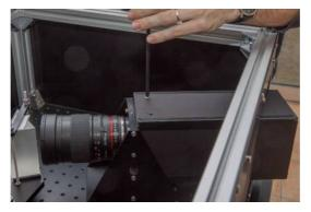
Install first the panel filler, using the counter plate with inserted nuts. Use 8 M4x10 screws.
