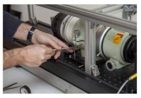
Note : You can move the slit& fiber image vertically either by rotating the camera module around a vertical axis, or by rotating the telescope #2. The best result is achieved when :
