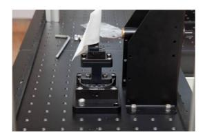
Use M6x16 screws (with plate washer & spring washer).
