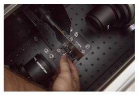
The tuning is quite easy to do : for a given stable light source (LEDs, for instance), stable from one image to the other, you can measure the max light level in the CCD image. The tuning is optimal when the light level is the highest.
