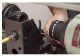
This mask has two functions. The first (main) one is to reduce as much as possible any parasite light (specially reflections around the input mirror). The second function is to make visible the nominal position of the optical axis to help with the alignement of both telescopes, and prevent any vignetting.
