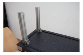
Then, put the 4 parts 210mm long like on this picture (with the bracket atthe righ position) :
