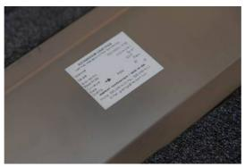
Slide the grating inside the mobile holder, with the blaze direction towards the open end of the holder. The grating surface must be towards the roof. Make sure, during the sliding that the grating surface is never in contact with the 3 screw heads above the surface :
