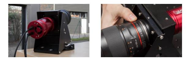
Take a special attention to this focus operation : it is critical for all following steps. The tuning is *very sensitive*. Do this operation in bin 1x1, with displaying the image at scale 1:1 (one screen pixel = one CCD pixel). Below, you can see the image (right) taken by the camera in the actual position (left).
