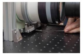
The fiber image size sould be the same as with the telescope #1 (because we've added a symmetrical system). The FWHM should be around 3,9 pixels (Atik 460EX).
