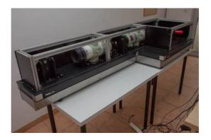
Next is the fiber side cover. Remove the fiber from the connector, and put the cap back on the connector. Make sure to not force on the fiber connector holder when assembling the cover.
