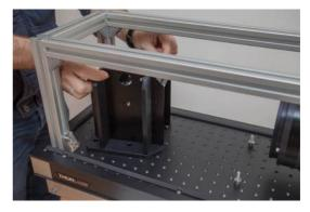
Use two M6x16 screws, with a flat washer and a spring washer for each. Do not tigthen the screws yet.
