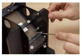
Put the tuning beam above the grating with four M3x8 screws.
