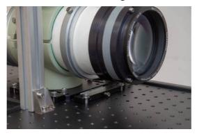
Put the CCD camera (with the lens) in front of the telescope #2. Check that both optics are well aligned.
