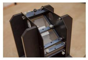
Put two M4x8 screws inside the grating holder (one on each side).
