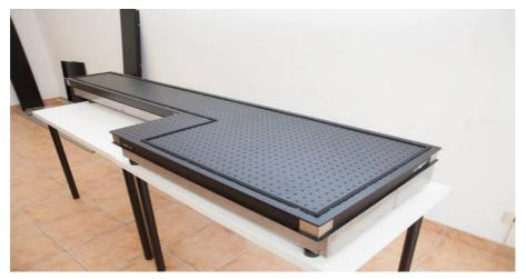
Next step is to install the cover structure. It is made of Bosch profile elements, with different lengths. Bosch profiles are attached to the optical bench with special brackets (left). Bosch profiles are attached together with Bosch standard brackets (right). Screws are M5 for the Bosch profiles (Bosch screws), and M6 for the optical bench. In the Bosch profiles, you can slide the nuts until you tighten the screws.
