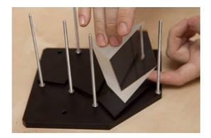
On top of each prism, put a small piece of soft material, and add the prism retainer. The soft material is there to prevent any damage on the prism when tightening the prism retainers.
