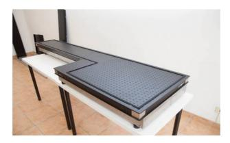
The mechanical structure is made of 9 U-shape stainless sheet metal parts.
