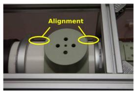
Use two tuning tools to guide the plate on both sides (attached with 2 M6x16 screws + plate & spring washer each).
