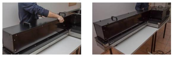
At the junction of the two top covers, place the top mask, with three thumb screws. The function of this mask, of course, is to eliminate any light leakage coming from the top.
