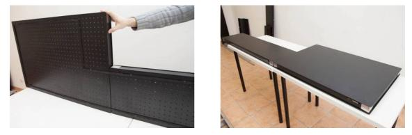
Mount the structure on the two benches, and attach each of them with 4 M6x10 screws (with spring washers). Before tightening the screws, make sure that the two optical benches are in contact, perfectly aligned. Tighten all the screws.
