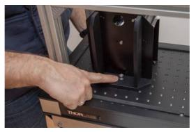
Install a tuning tool, in front of the grating base : it will help you to make a precise rotation of the grating in the next step.
