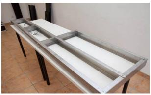
The whole structure is mounted with M6x12 screws (each screw with a spring washer and a nut). Assemble the long elements first, with the 4 short crossing parts. Then, add the side part with 2 long crossing parts. Warning : the long beams are not symmetrical ; make sure that they are matching properly.
