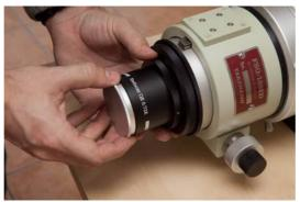
The gap between the focuser body and the first black ring must be 12mm : tune this position with the telescope focuser, and tighten the focuser (bottom lever). The Takahashi focuser will not be used anymore.
