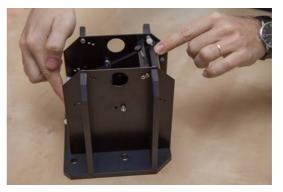
Now, let's install the grating in the mobile part. Put it on the table, with the plastic screws toward the table.
