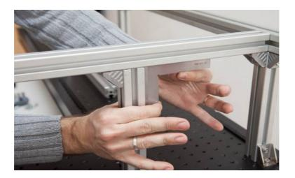
Then, put the last long element (1320mm), like on the picture. Use the precision steel set square to make sure the angle is right. Check that the outside width is 230mm.
