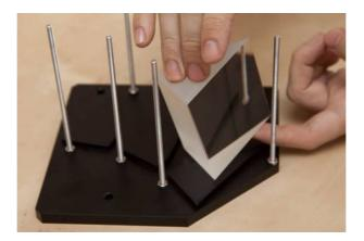
The prisms holder is made of the plate, three legs, three prism retainers and six threaded rods (120mm long).
