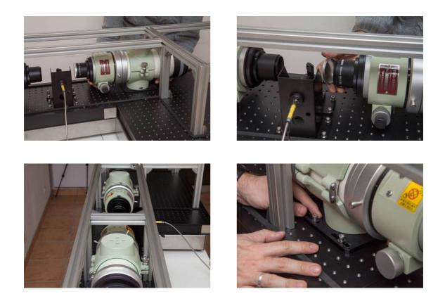
Use two tuning tools to guide the plate on both sides (attached with 2 M6x16 screws). Use a third tuning tool to make a fine focus tuning (attached to the bench with two M6x16 screws, and using a M4x40 screw for the tuning)
