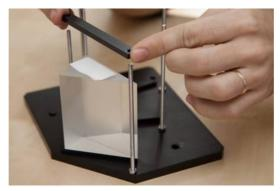
Add a nut, with three spring washer on each threaded rod, and gently tighten them. The prism must be strongly attached to the plate – but make sure that there is no risk to break them (do not tighten too much – it can be tighten by hand).
