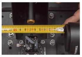
Make sure that the lense axis is exactly parallel to the bench edges (visual control is enough).
