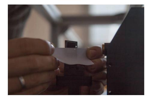
If the spot is not properly positionned (1mm frm the mirror edge and 102mm from the optical bench), untighten the whole module (input mirror), and slightly correct it – then re-tighten the screws.
