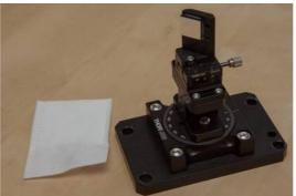
The input mirror reflects the light coming out the fiber at 45°, towards the long axis of the instrument. The optics inside the fiber module makes a transportation of the fiber image on the input mirror. The mirror can be tuned precisely (horizontally and vertically) to make sure that all the light is going in the instrument (no vignetting effect).
