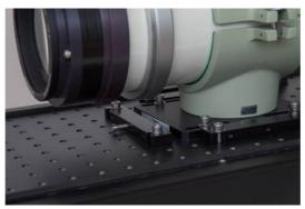
Put the CCD camera module in front of the telescope (where the grating module will take place afterwards). Check that both optics are well aligned.
