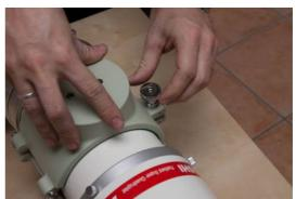
Install the Takahashi focal reducer (x0.73) on the telescope. The gap between the focuser body and the first black ring must be 12mm : tune this position with the telescope focuser, and tighten the focuser (bottom lever). The Takahashi focuser will not be used anymore.
