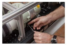
At this stage, you've made the most critical alignement : the beams coming through the two telescopes are perfectly aligned. You now have simply to add the two dispersers (main grating and prisms) to spread out the light coming out from the fiber.
