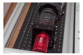
Switch on the source light in the fiber and acquire images from the CCD camera : you should see the fiber image, and the whole mirror.
