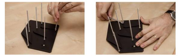
Put each prism at its exact position (given by the shape machined in the plate). Never put a finger on the polished surfaces ; take the prisms only by unpolished surfaces.
