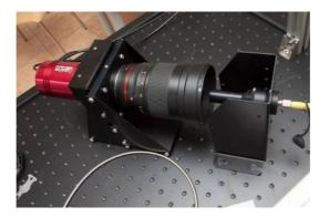
The camera lens is focused at th infinite. And the lens inside the tube should be focused on the fiber input. Then, you should see the fiber image pefectly sharp in the CCD image. You can calculate the expected FWHM for the image : the fiber is 50 $\mu$ , and the first afocal lens is 30mm, and the photo lens is 135mm. Then fiber image on the CCD is 50 x 135 / 30 = 225 $\mu$ . If the pixels are 4,54 $\mu$  (Atik 460), the image size must be 50 pixels when perfectly focused.
