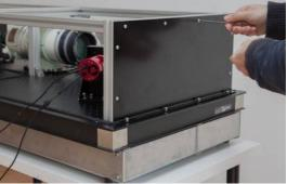
Third panel is the intermediate one, beside the telescope #2. Do not put the two screws in the vertical element, close to the telescope. They will come with the fiber panel.
