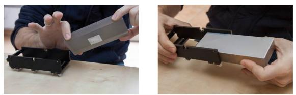
Assemble the grating closing beam, with two M3x12 screws. Before assembling, check that the tuning plastic screws are cleared out.
