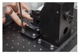
The remaining M3x6 screw (the last one in the screws bag) is made to attache (later on) the mask ; you can put it in place on the mirror holder temporarly.
