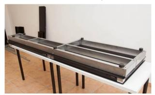
When the structure is finished, return the whole optical bench : you now have the reference surface for the whole instrument.
