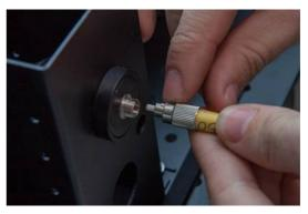
Make the spot coming out the fiber is focused on the mirror, about 1mm from the edge, and at mid height of the mirror vertically (102mm from the optical bench surface).
