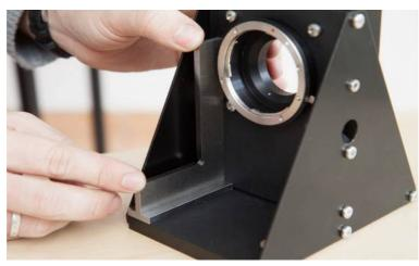
Assemble camera & objective lense on the holder, making sure that the optical axis is perfectly parallel to the base plate.
