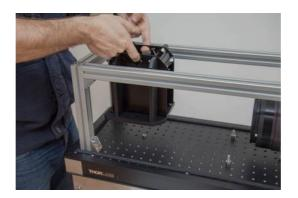
The module must be free to rotate around the M6 screw. Let it in a nominal position (parallel to the optical bench)
