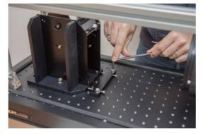
Switch on the light source in the fiber and acquire images from the CCD camera. You can see the wide slit in the mask, but probably not the spectrum itself, which is dependent on the grating holder rotation.
