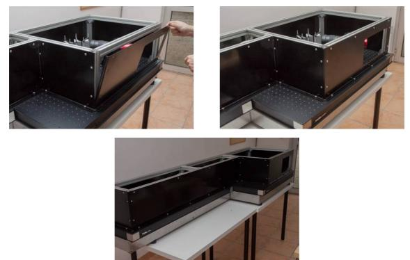
The camera cover has a large opening, to adapt to the camera holder. You can simply put a filler in the opening, with a small hole for the cables (power supply and USB). But it is better to make a tube (with carton box, for instance) around the camera, going out the sidecover : this way, the cooling of the camera is not interfering with the air inside the eShel+ cover, and the temperature is more stable.
