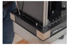
When screws are tightened, they press the gasket and prevent any light leakage, and make the top holes of the cover side in front of the Bosch nuts. When pressed, the gasket must be 2mm thick. Then, put a screw in each remaining hole in the cover, and tighten them.
