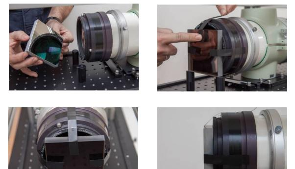
Switch on the source light in the fiber and acquire images from the CCD camera : you should see the fiber image (like with the telescope #1), and the whole mirror... two times ! (one from the front, and the other from the rear - symmetrically).
