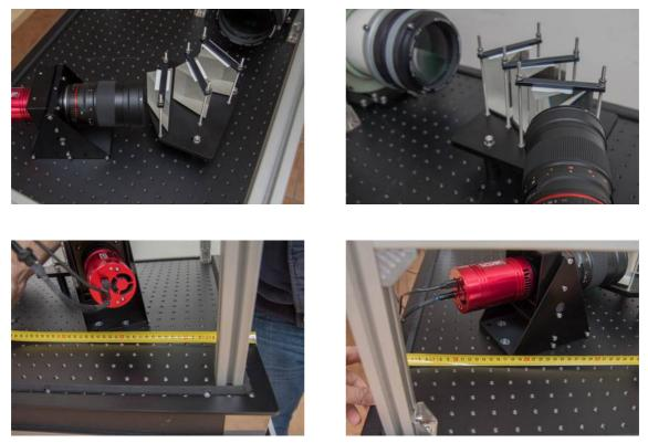
Put four (at least two) M6x16 screws, with a M8 flat washer, an M6 flat washer and three M6 spring washer each. Do not tighten the screws right now (holes are big enough to make some adjustments of the position).
