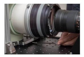
Then, tighten the telescope #2 plate on the optical bench.
