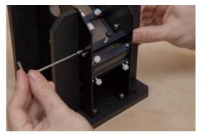
The grating holder is done ; you can precisely tune the grating angle with the two thumb screws.
