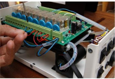
Add the complementary red wire (provided in the upgrade kit) as follow (between pin #NO2 and #NO4 on the PCB) :
