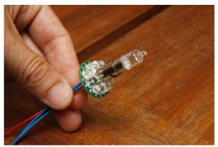
Mount the electronics in the new ring (provided in the kit) :
