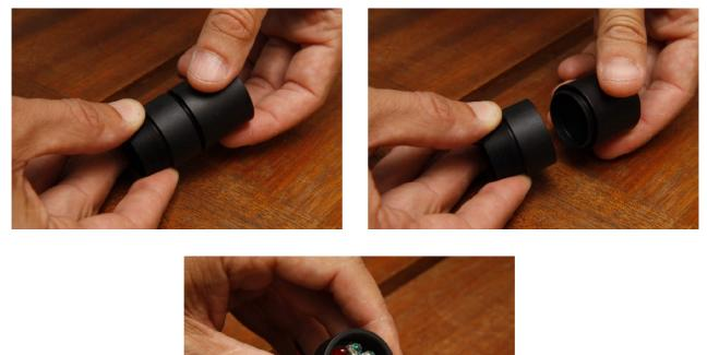
Unscrew the retaining ring of the electronics. You must do several turns, using the slits made in the ring:
