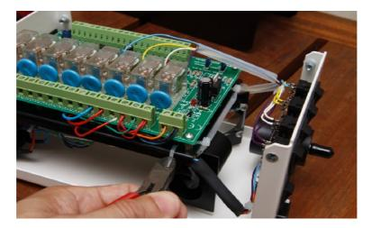
Unconnect the 2 wires of the Flat Module
